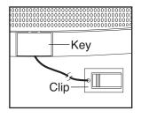
a moment, the displays will light. IMPORTANT: In an emergency situation, the key can be pulled from the console, causing the walking belt to slow to a stop. Test the clip by carefully taking a few steps backward; if the key is not pulled from the console, adjust the position of the clip.
